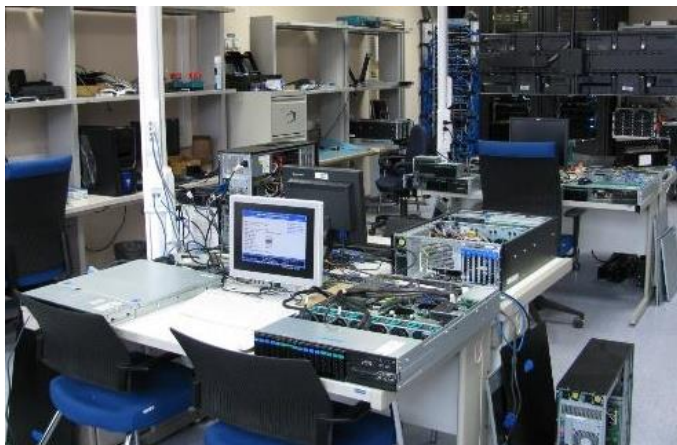
PCSD systems are checked out for stress testing, issues replication and components compatibility sanity check
