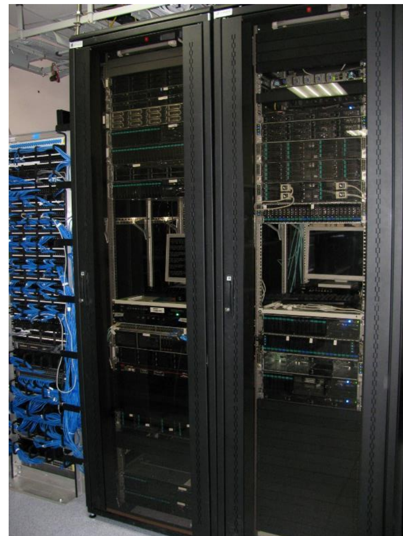
Cluster for performance scaling, power and thermal evaluation as well as testing of configuration and software tools.
