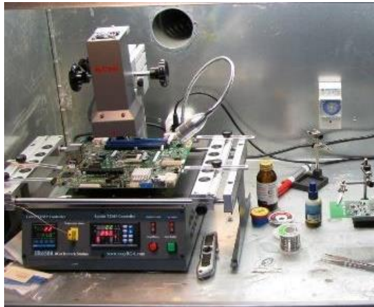
BGA rework station for complicated CRB rework (SPI flash, chipset, CPU socket soldering/unsoldering work)
